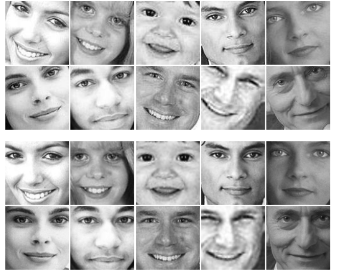
Fig. 2. Pose correction using TILT. Top rows: original face images with rotations ( \tilde{F} ); Bottom rows: corrected face images ( F ).
