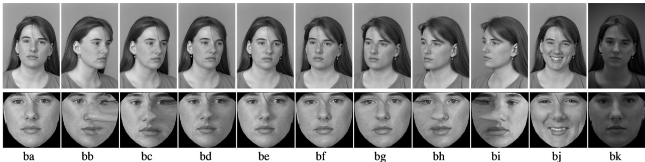
Fig. 9. Face images of a sample subject from FERET b-series database (upper row), and their normalized faces (lower row).
